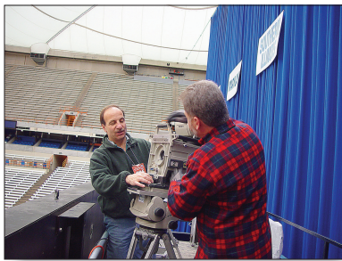
Figure 2.83 Next the camera head is slid into a V-shaped wedge plate on the top of the pan/tilt head and locked into position with a lever that pushes a pin into the camera's base from the wedge plate.
