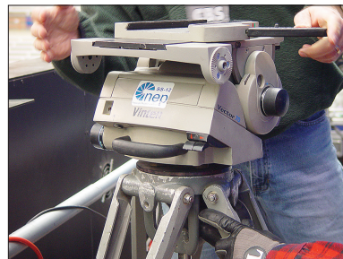
Figure 2.82 Next a pan/tilt head is mounted. The bottom of the head has a threaded column that is keyed and mates with an opening at the top of the pedestal. An inside threaded ring, usually brass, is screwed on from inside the pedestal (where the gloved finger is pointing). These heads are about as heavy as the tripod. They have a counterbalance mechanism to provide up to \pm 60^\circ balanced tilt range for camera, lens and teleprompter combinations weighing up to 154 lbs.
