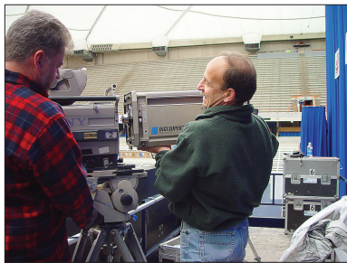
Figure 2.84 Then the zoom lens is mounted. It literally hangs on a thin, inverted V-wedge plate along the top front of the camera. Gravity, via the leverage of the heavy lens extending out from the camera, forces the bottom of the lens to firmly push against the camera. To play it safe a small knob extending from the bottom of the camera controls a quarter turn plate that the tab extending from the rear bottom of the lens fits into.
