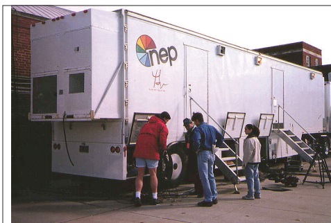
Figure 2.75 Although a crew is made up of people with diverse talents, those involved with remotes often help with common tasks. Once the truck is parked, an early task is to run the necessary cables. Most of the crew is involved. (Source: Tim Stoffel)
