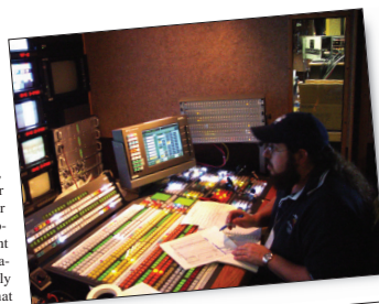
Figure 2.85 TD loading effects into switcher based on input from the director and other production staff. The video switcher is taught the sources to select and manipulate during the effect. A single effect can have multiple transitions and actions, each anchored as a keyframe. Each keyframe is loaded manually the first time, and a timeline is entered as to how much time will elapse between successive keyframes. Then the whole effect is stored. Now, the push of a single button — or even an external event, such as a flag signal from an official's box in a sporting match — can run the effect. Most effects do not have to be built from scratch, as the client's production department will often bring them on disk or even download them over the Internet straight into the switcher and DVE/DME. In addition, keyframes from one effect can be used to build a new one.
