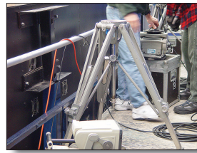
Figure 2.81 Building a camera starts with a base for the camera, called a pedestal. The legs are adjustable to change the height. To support the weight of a camera, most early pedestals had steel legs and a cast-iron frame. Today aluminum, and even carbon fiber, are used to build tripods designed to support 200 or 300 lbs. Early tripods weighed over 50 lbs — today's are down around 30 to 40 lbs.
